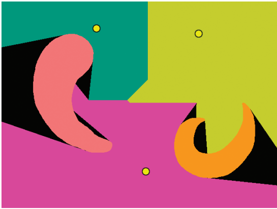
14 Running three simultaneous box-visibility fills. Notice that the fills interfere with each other and that their boundaries are all on 45-degree lines.
