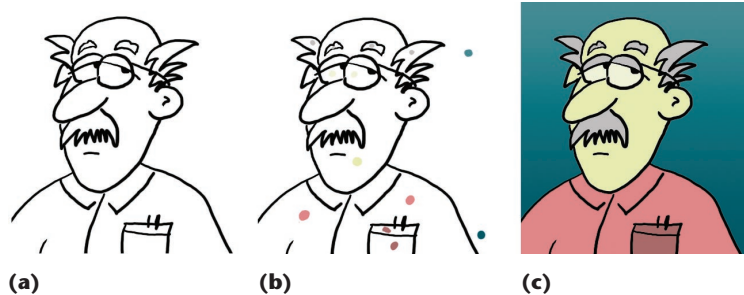
1 The classic flood-fill algorithm for cartoon cels. (a) A line drawing. (b) The color scheme indicated by dots. (c) The result of filling each region.
