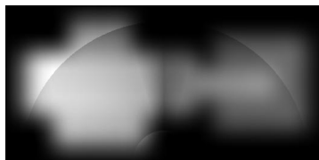
6 The cost pattern C_S = D \times B(S) . This results from weighting the wiper density, then scaling each point by the driver's windshield importance.
