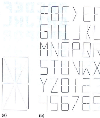
4 (a) The 16-segment display. (b) The alphabet and digits. Note the really lame B.
